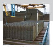
钢管与吊带可以贮存在一起. 不需要再重新吊装 The product stored with the sling. It is **not necessary to resling**.
