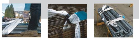
The sling is only placed once in the transport process. The product is carried throughout the factory with the same sling.
